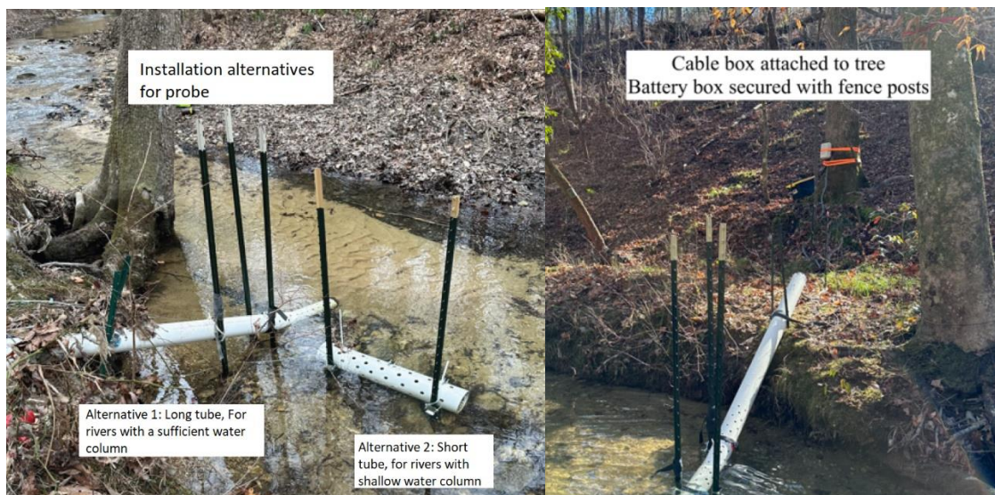
Picture 1. Left: Alternatives for probe installation in the stream. Right: Cable, battery container and box attached to the tree.
